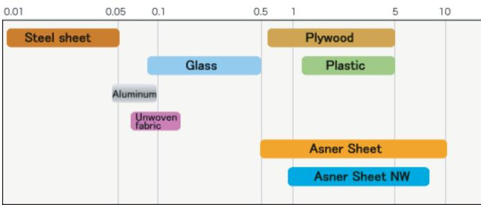
Loss coefficient n was measured on a laminate with unwoven fabric, for example, sandwiched as a damper between aluminum sheets.
